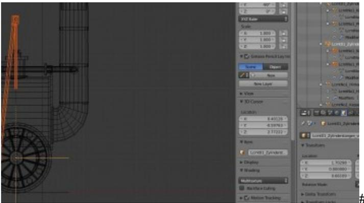
Then turn the entire group about its center (=the wheels axis) so that the piston rod lies in parallel to the x axis. Note the angle well, then run "Apply Rotation" on the entire group.
