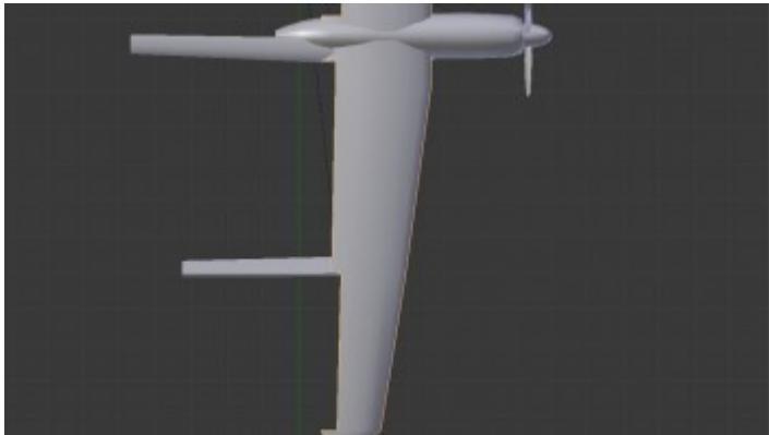
In order to do so, we enter the Object mode and add another part to the model. This part will be the cutting template and will have Blender cut along its edges. Precisely. Of course, the circle here is just an example; it is absolutely possible to use highly complex shapes as well if so desired.
