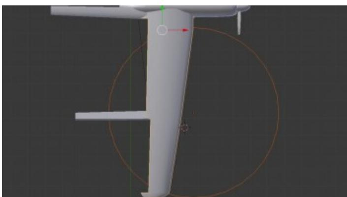
So we can now proceed to enter the Edit mode. Unmark all the parts of the object to be cut, then click "Knife Project". Blender will now project the template on its recipient along the line of sight and slice it precisely where the projection meets it. It will either cut only the surface or all the way through, depending on whether "Cut through" is activated or not.
