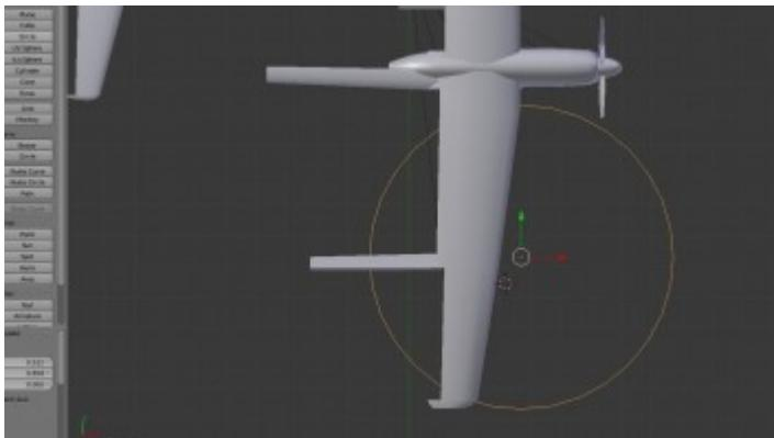
Now we need to tell Blender that this circle is the template to cut along and that the wing is the part to be cut. This is rather simple: first mark the circle, then with Shift pressed, select the wing. Everyone has seen this already: now the circle is the orange reference part and the wing is marked yellow.
